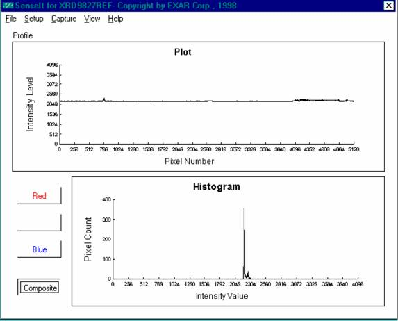
Figure 5. Non-calibrated Black Target Scan
